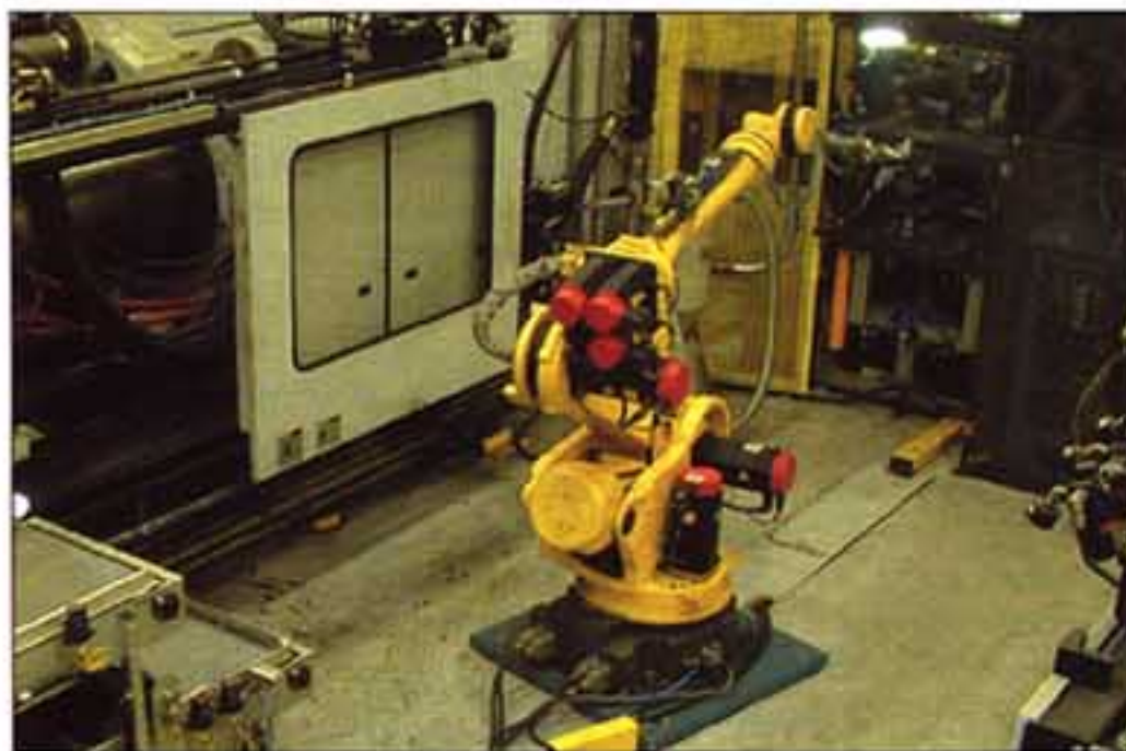
A single robot can empty two 750-ton injection-moulding machines.
